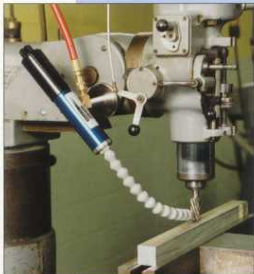
The Model 610 Adjustable Cold Air Gun is ideal for cooling milling operations.
