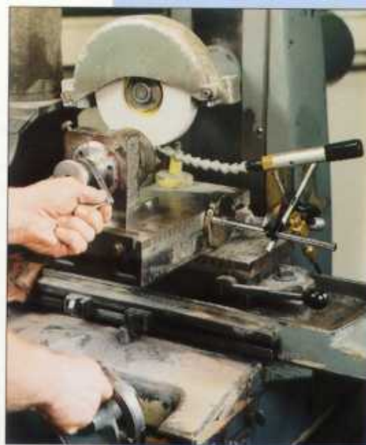
Model 608 Mini Cold Air Gun cools dry surface grinding operations for reduced production times.
